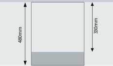
Bed hole with 150mm of type 1 infill
