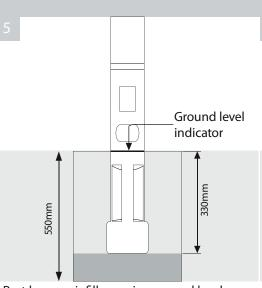
Rest base on infill ensuring ground level indicator is level with ground. Orientate so that red reflective panel faces into direction of traffic flow
