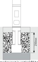
Ensuring marker post is vertical fill hole with C20 concrete mix until 100mm from ground level. Once concrete has cured return final wearing course to ground level
