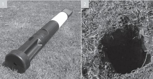
The reflex verge marker base is concreted to give Dig 450mm square and 480mm deep stability during flexing. The moulded return on the base ensures the marker cannot be removed
