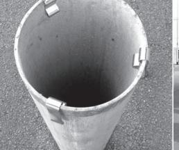
the top edge of the core. Ensure the long leg of the clip is located on the outside of the tube
